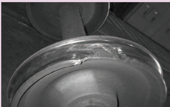
Photograph of a damaged train wheel
