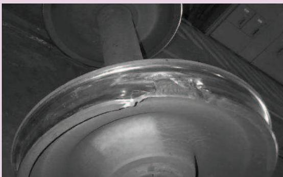
**Photograph of a damaged train wheel**
