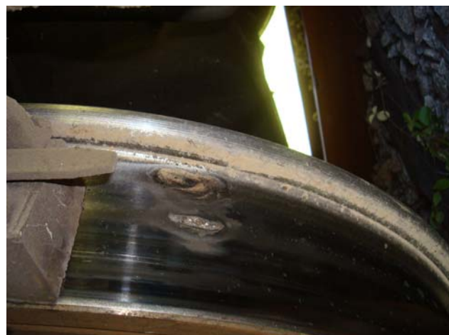
Figure 1 Damage on a wheel due to breaking
