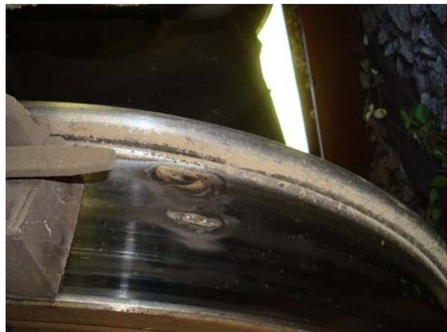
**Figure 1** Damage on a wheel due to breaking
